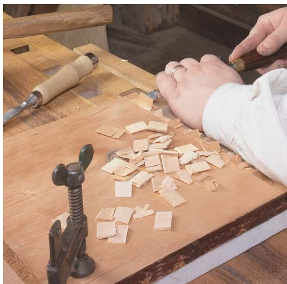
▲ Routers, dovetail bits, and dovetail jigs didn't exist in 1875, so cabinetmakers relied on more traditional methods for creating dovetail joints. First, John lays out the dovetail pins with a pencil and cuts the sides of them with a hand saw. Then, he removes the waste between them using a chisel ( Photo above ).
