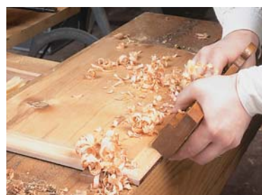
▲ Planes handled many shop tasks in 1875. Here, John adjusts a jointer plane ( above ) and rounds an edge with a hollow plane ( below ).
