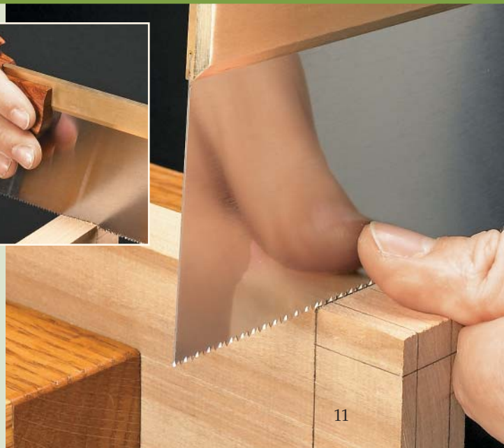
▲ Conventional handles may work well for framing saws, but they don’t offer the control needed for fine joinery work.
