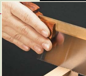
▲ Conventional handles may work well for framing saws, but they don’t offer the control needed for fine joinery work.
