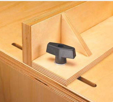
▲ Router Fence. Grooves in the router table allow you to easily position the fence and lock it securely to the tabletop.
