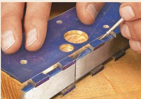
7 With a spacer block, hold the two sole blanks between the sides. Then scribe the pin profile on the sole blanks.
