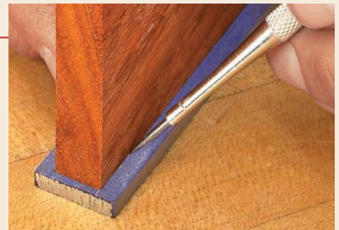
5 After centering the infill blank on the sole piece, you can scribe the baselines for the dovetails.
