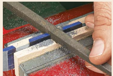
8 Once you rough out the waste to form the pins (like you did on the tails), finish up with fine needle files for a tight fit.
