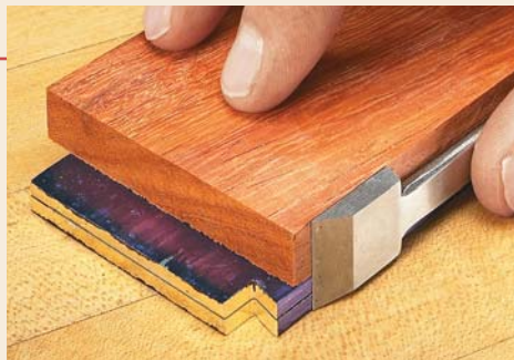
4 Using the plane iron as a gauge, plane the infill stock down until the plane iron matches the width of the iron.
