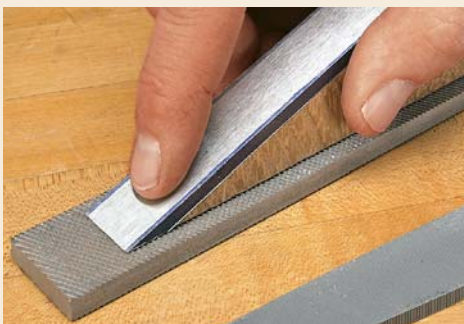
6 Use a wood guide, cut to match the bed angle, to file the 20^\circ bevel on one end of the long sole blank.
