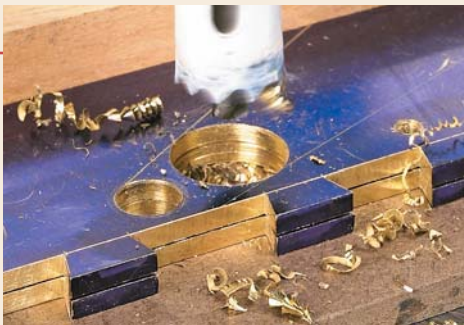
3 I used a \frac{3}{4} "-dia. hole saw and \frac{7}{16} "-dia. bit to rough out the mouth opening. Then drill \frac{3}{16} "-dia. holes for the rivets.
