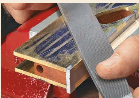
6 A flat file smooths the sides and sole. Just be careful not to round over the edges of the plane body.
