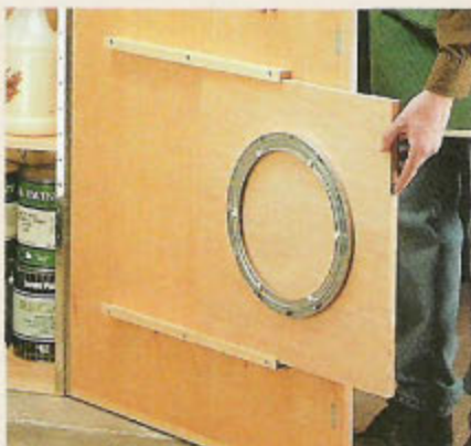
B. Lazy Susan. When the lazy Susan is not being used with the work table, it stows away inside the cabinet.
