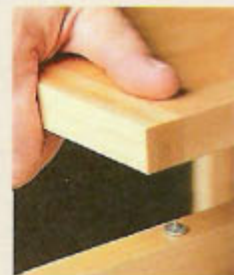
A dowel center makes it easy to locate the hole for the steel pin in the bottom of the work table.
