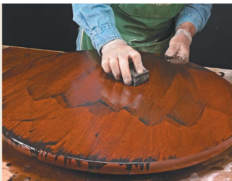
▲ Under the messy paste formed by the oil and the brown rottenstone powder, the finish is taking on its final mirror-like gloss. I put in a little extra time at this stage.
