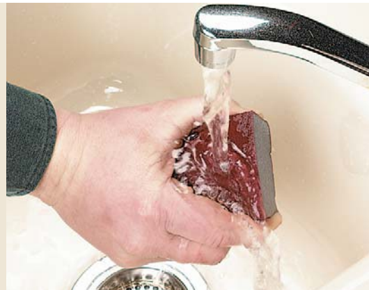
▲ When foam sanding blocks or sponges get loaded up with sanding dust, you can rinse them out in water and reuse them when they are dry.
