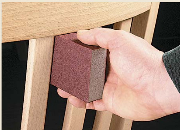
▲ Another feature of foam sanding blocks is that there's abrasive on four sides for getting into tight places.
