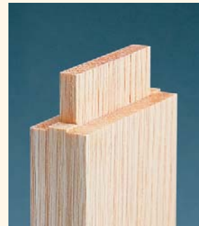
Stepped shoulders on a tenon indicate that it's time to give the rip fence a little tune-up.
