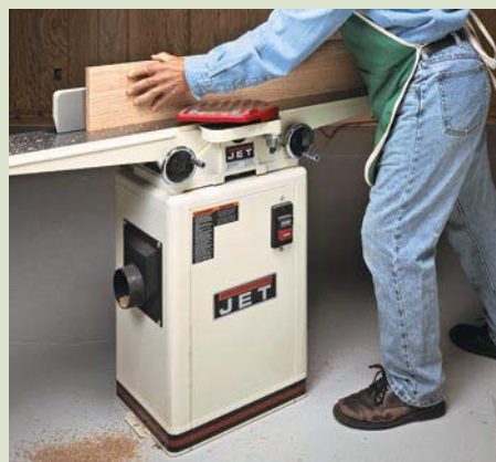
▲ Keep pressure on the leading edge of the workpiece as it passes over the cuthead and onto the outfeed table.
