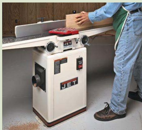
▲ The left hand applies the downward force and also keeps the workpiece tight to the fence.
