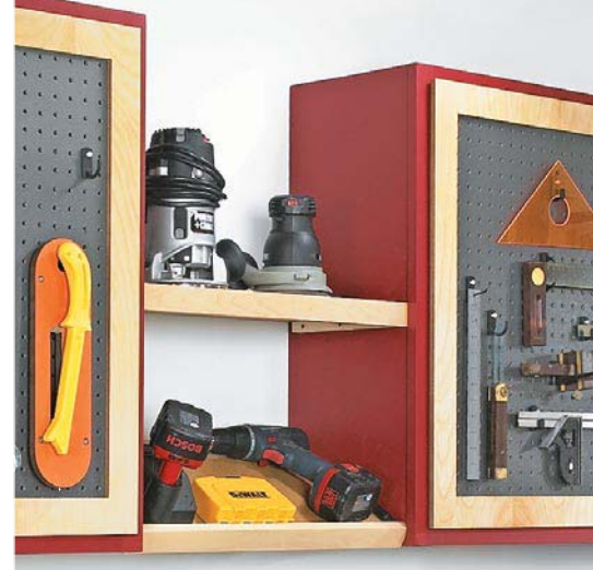
The upper shelves can be mounted level (with the front edging facing down) or at an angle (edging up).
