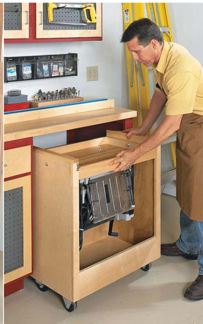
The “flip” top on this cart makes it easy to set up the planer for use (left) or stow it underneath for compact storage (right).
