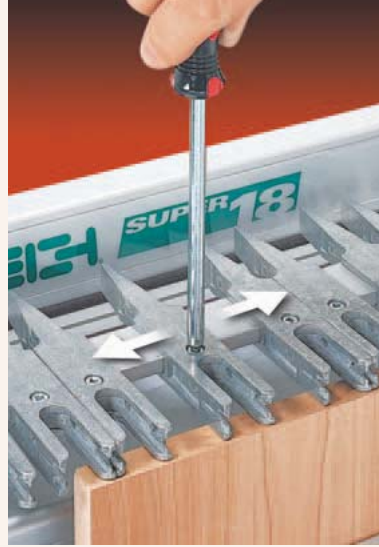
▲ Fingers. To customize the size and spacing of the dovetails, just slide the fingers into position and lock them securely in place.
