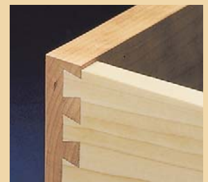
Offset. If the pieces don't align at top or bottom, they may not have been tight against stops.
