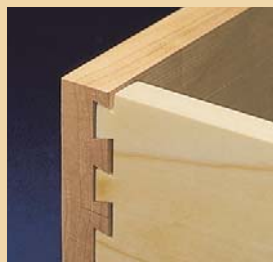
Too Loose. If joint is too loose, increase bit depth.
