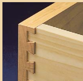
Too Deep. If pins go deep, move template forward.
