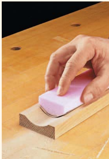
▲ A sanding block fashioned from a piece of foam insulation makes quick work of sanding the cove.
