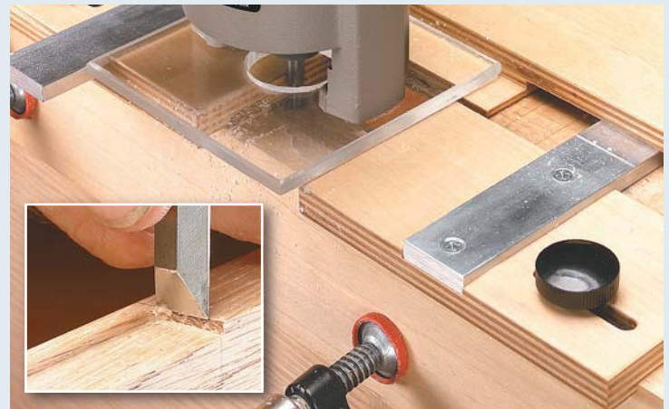
4 To remove most of the waste, rout clockwise around the inside edges of the aluminum guides and back stop. Then using the mortise as a guide, square up the corners with a sharp chisel (inset).
