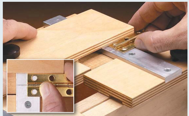
2 Here again, you can use the hinge to set the width of the mortise. A typical installation is to adjust the back stop until the centerline of the knuckle lines up with the scribe mark (see inset).
