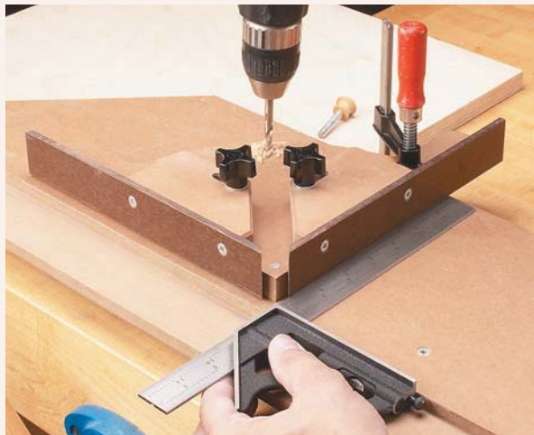
2 To drill the two holes for the right angle settings, reposition the stop so it is square to the front edge. Countersink the holes after drilling them to make it easier to insert the locking pin.
