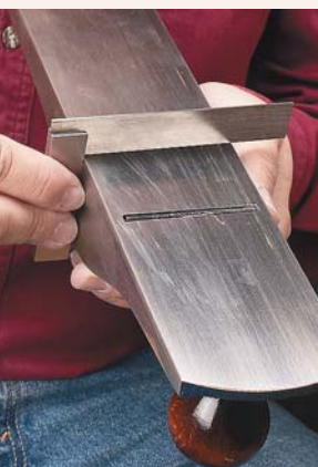
▲ Check for Square. To get good results, the sides of your plane need to be square with the sole.
