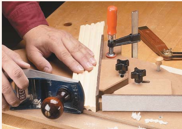
▲ Other Angles. By disengaging the locking pin and securing the stop block with a clamp, you can use the shooting board to trim miters at any angle.
