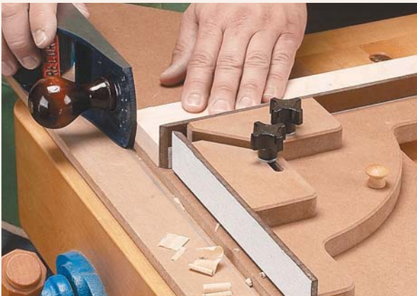
▲ Shooting End Grain. With the stop block set perpendicular to the edge of the shooting board, you can shave a hair off the end of a workpiece.
