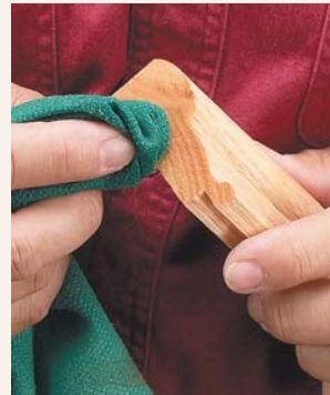
▲ Smooth Cutting. Dampening the end grain with a wet cloth makes it easier for the plane to slice through the wood without tearing the fibers.
