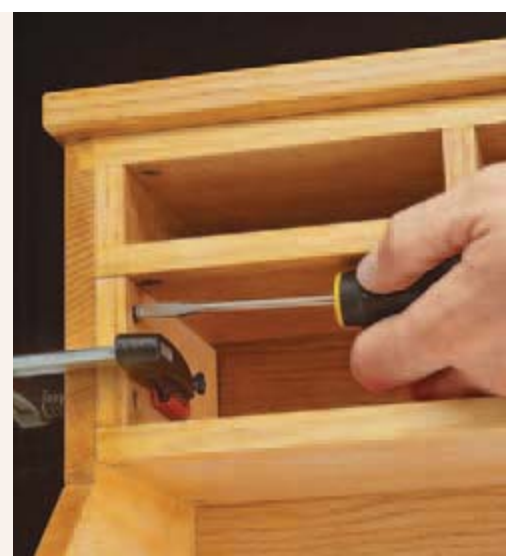
▲ Lower Bay. A few screws in the sides fasten the lower drawer bay inside the case.
