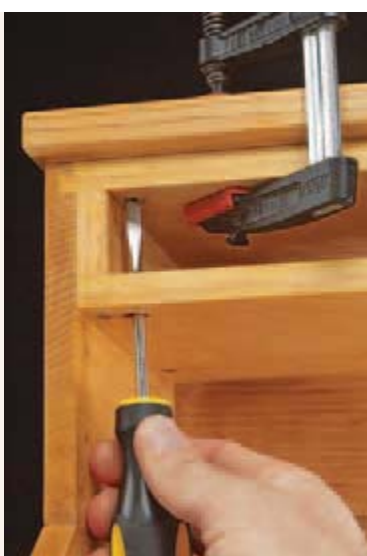
▲ Attaching the Top. Access holes in the upper drawer bay let you screw the top in place.
