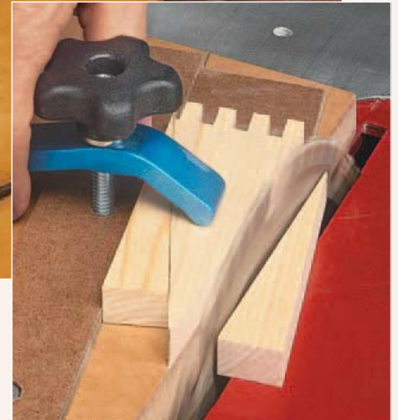
▲ Wedges. The trick to cutting the pie-shaped side pieces for the curved lid is the jig you see at right. (For more, refer to Shop Short Cuts on page 34).
