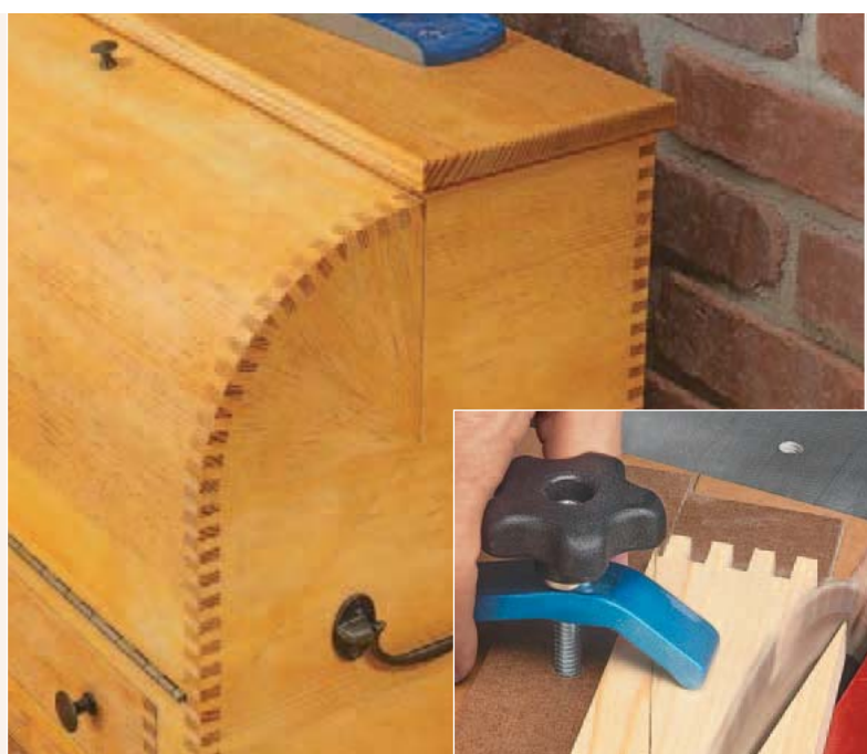
▲ Wedges. The trick to cutting the pie-shaped side pieces for the curved lid is the jig you see at right. (For more, refer to Shop Short Cuts on page 34).
