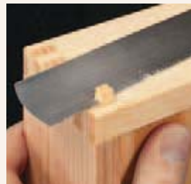
▲ Plugs. Endgrain plugs hide the gaps left from cutting the rabbets and grooves for the drawer bottoms.
