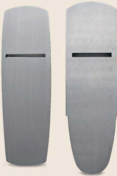
▲ Sole Difference. The sides of the Veritas plane (right) are machined square to the sole.
