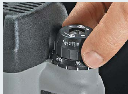
▲ Micro-Adjust. A micro-adjust dial provides an easy and accurate way to fine-tune the depth of cut.
