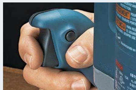
▲ A Handy Switch. You won't have any trouble finding the trigger switch on the handgrip of this plunge router.
