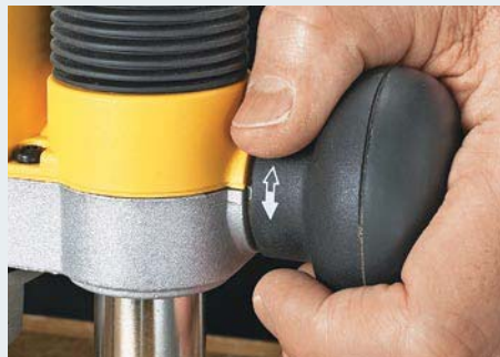
▲ Grip Plunge Lock. Turning the handgrip on this plunge router locks and unlocks the plunge action.
