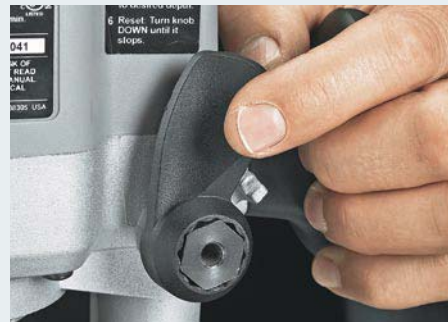
▲ Lever Lock. The most common type of plunge lock is a spring-action lever. You pull it back to release the lock.
