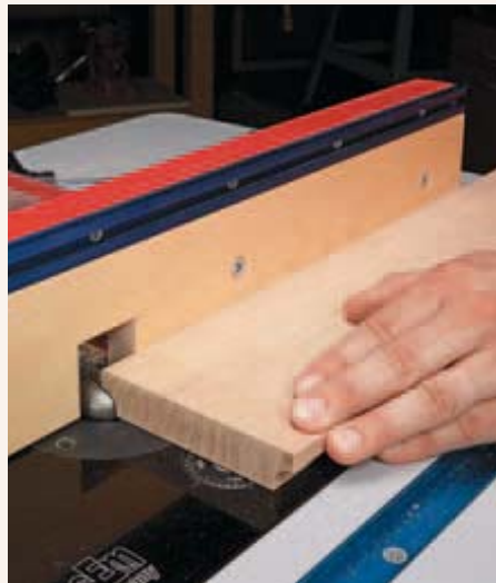
▲ Start Wide. It’s safer to rout a profile on both edges of an extra-wide blank. This gives you more control and keeps your fingers away from the bit.
