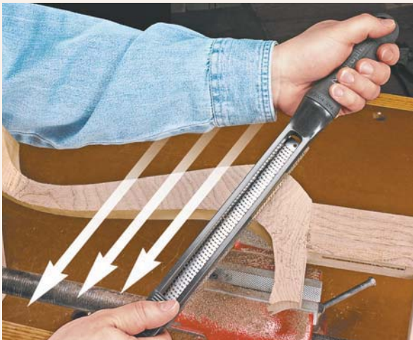
▲ Pull Stroke. If you get tearout from the previous motions, try reversing the direction of the rasp. Flip the tool end for end and pull it toward you to cut.
