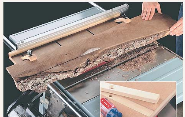
Ripping. To rip a straight edge on a rough board, just remove the runner.
