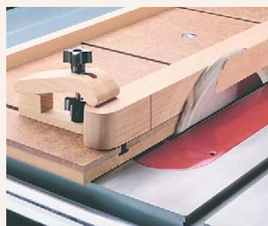
Step 6. After cutting a taper on one side, rotate the leg and repeat the process for each side.
