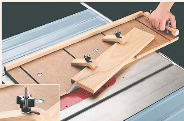
Angled Cuts. Two adjustable hold-downs clamp work securely in place when making angled cuts.
