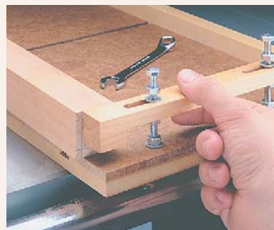
Step 3. Next, align the mark for the taper with the edge of the jig and tighten the adjustment nuts.
