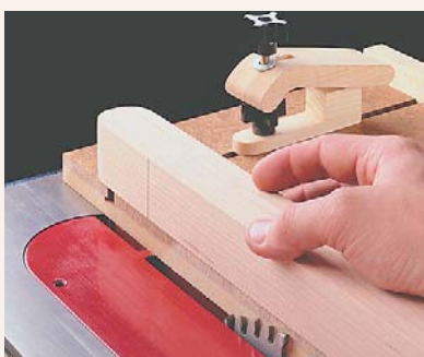
Step 4. Now lay out the starting point of the taper and align the mark with the edge of the jig.
