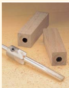
▲ This barrel trimmer squares the ends of the blanks to the barrels, so the pen mechanism will fit together without any gaps.
