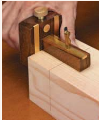
▲ Shoulders. With a cutting gauge, score the shoulders to establish the tenon length.
