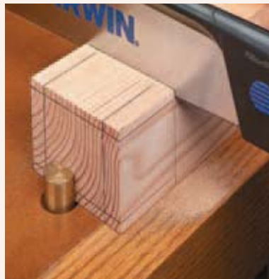
▲ Shoulder Cuts. Clamp the workpiece to the bench and cut all four shoulders.
