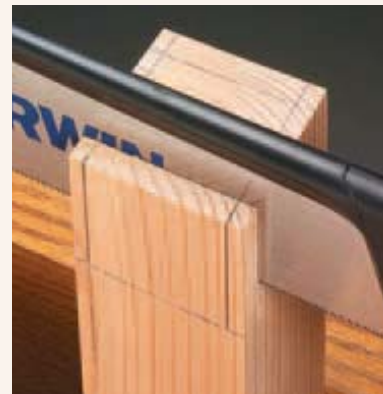
▲ Cheek Cuts. Level the saw to complete the cheek cut. Take it slow to avoid over cutting.
