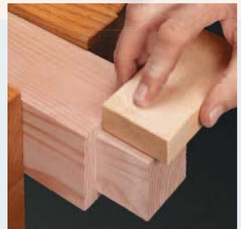
▲ Sanding Block. A hardwood block with sandpaper on one face makes quick work of fine-tuning the fit of the tenon.
