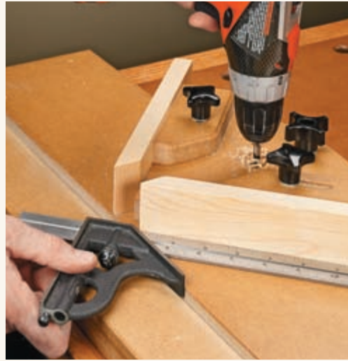
▲ Setup for 45°. After positioning the fence, drill a hole in the base using the hole in the fence base as a guide.
