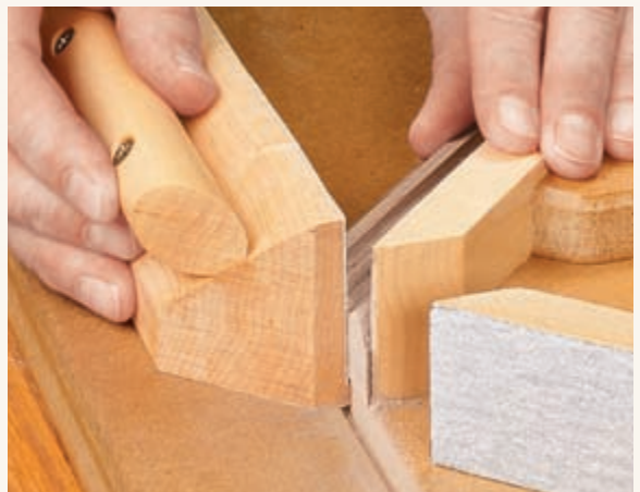
▲ Sanding Block. Another option for tweaking the fit of a workpiece is this shop-made sanding block. It slides along the base just like a hand plane.
